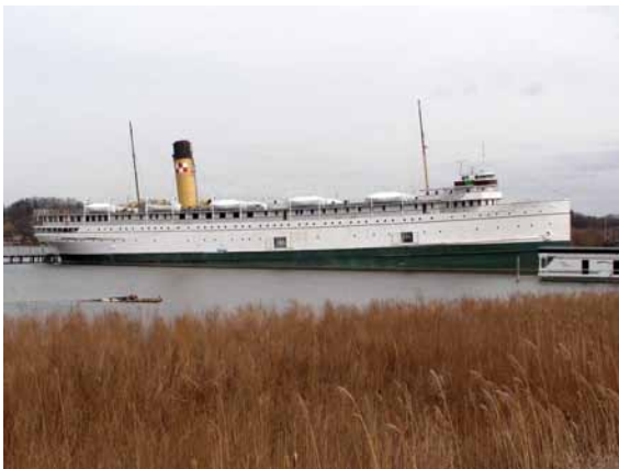
Here is another view of the SS Keewadin, moored at Douglas, Mi. Note the pilot house: originally there was no pilothouse; the wheelsman was out in the weather!
